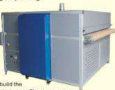
This electric tunnel dryer can apply to cure the garment after digital printing. It uses aluminum to build the frame, and set two blowers on the bottom to recycle the hot air. The temperature raise is very fast, 15mins to raise to 160°C, and it can cure the ink very well in short time.
