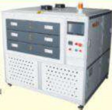
This box dryer with three drawers is applying for curing the digital printing T-shirt. Each drawer has the motor to drive its in and out. The blower and heaters is on the bottom of dryer. The hot air is running by the blower to cure the T-shirt through the hot air channel. The PLC controls the curing time and in/out of each drawer by the touch screen. The exhaust duct in on the top of the dryer, it can flow out the smoke during the period of curing.
