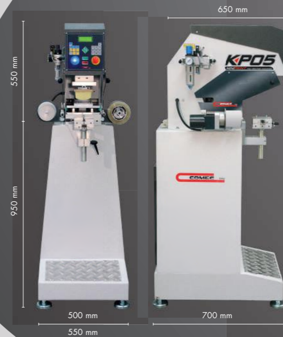
MINIPRINT KP05 1C with closed inkcup and ceramic ring Ø 90mm and steel bench
