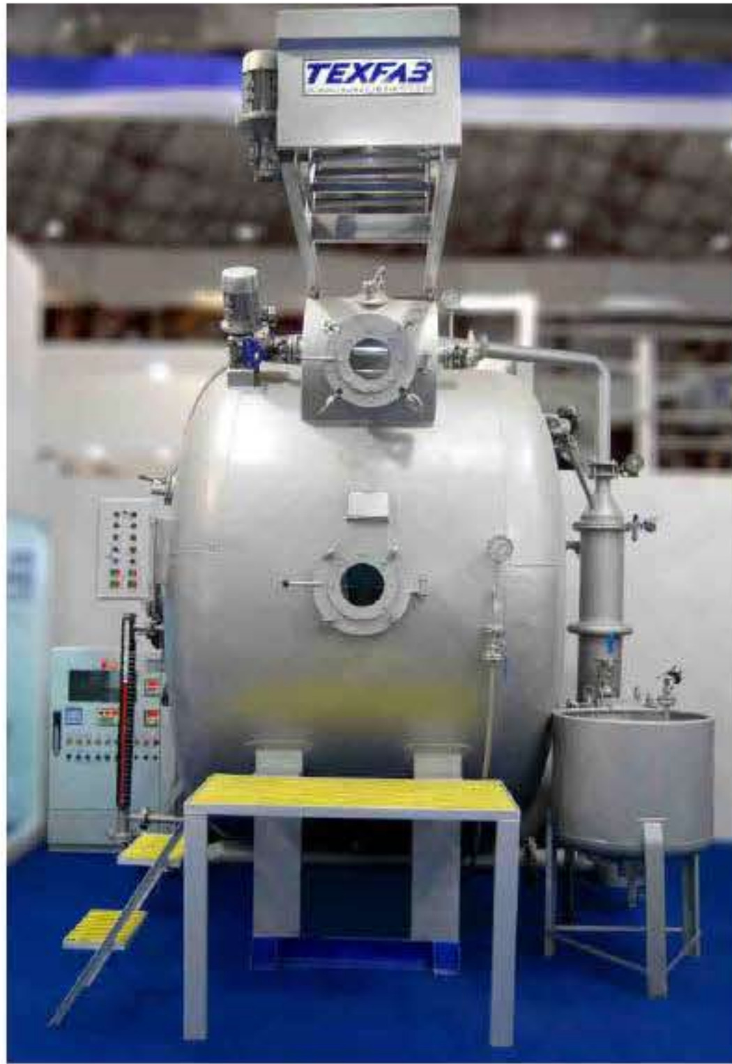
'O' Shape Sample Fabric Dyeing Machine Capacity available is 25 & 50 Kg
