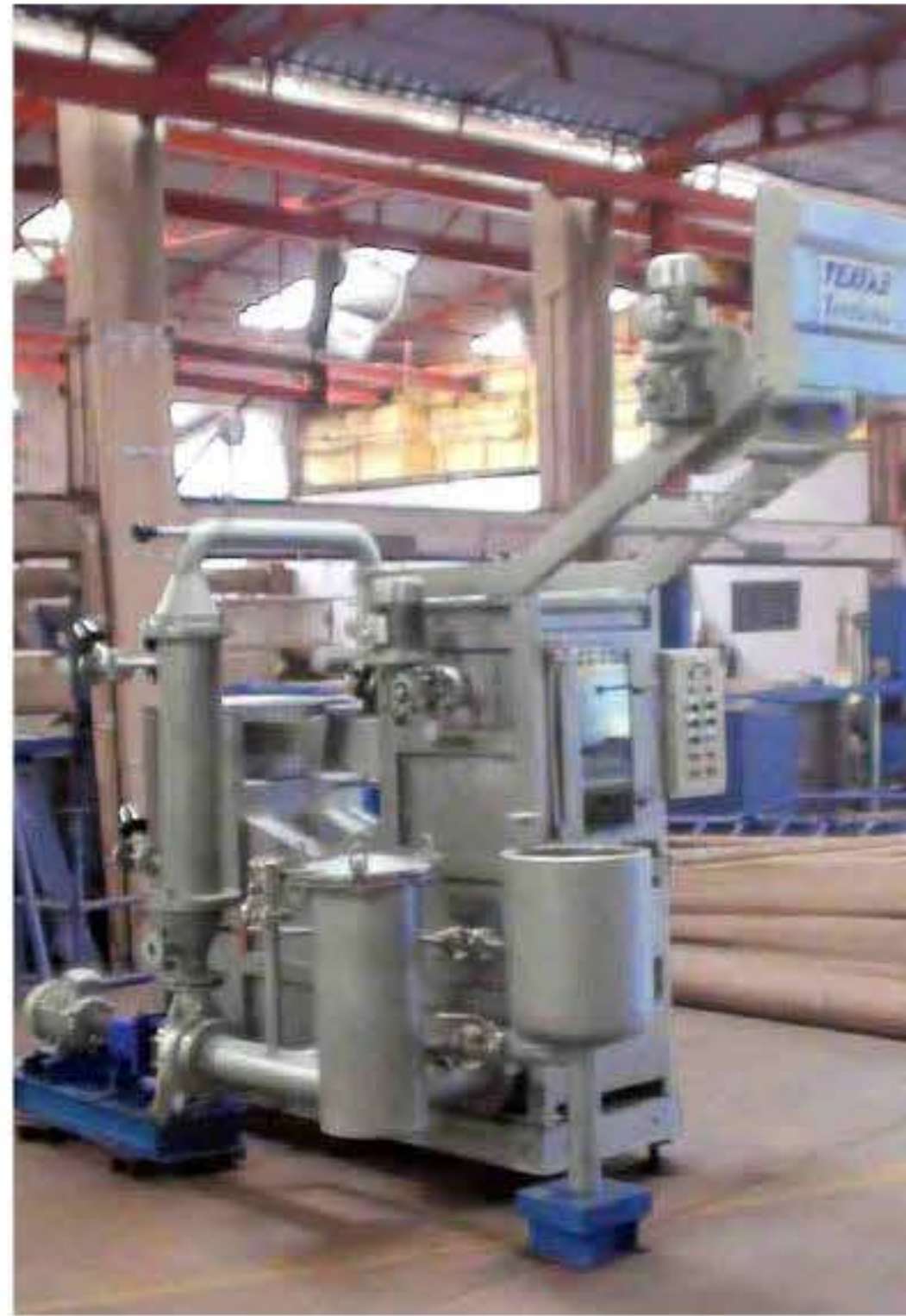
Terelena Caustic Soda Fabric Mercerizing Machine with Caustic Recovery Unit Capacity available is 50 Kg
