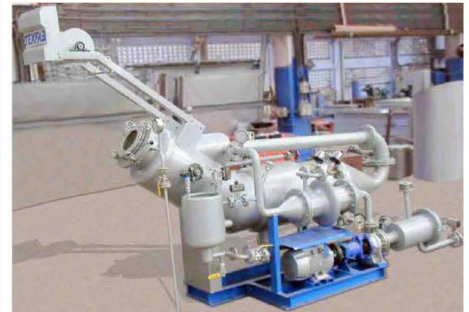
Sample Top Tube Fabric Dyeing Machine Capacity available is 10, 15, 20 & 25 Kgs
