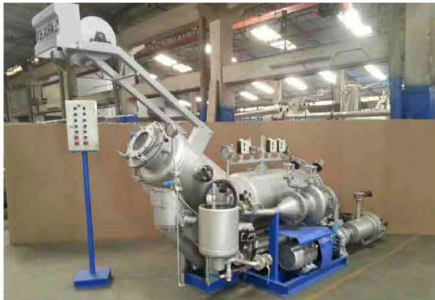
Sample Bottom Tube Fabric Dyeing Machine Capacity available is 10, 15, 20 & 25 Kgs
